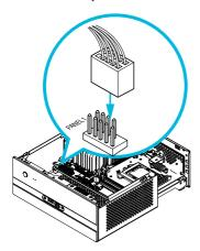
2. Connect the USB cable to the USB Header on the motherboard.
