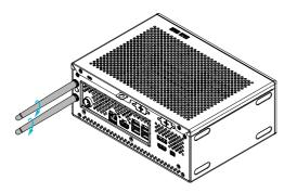
7. Turn the antenna clockwise until it is securely connected. Set the WiFi 2.4/5 GHz Antenna at 90-degree angle.
