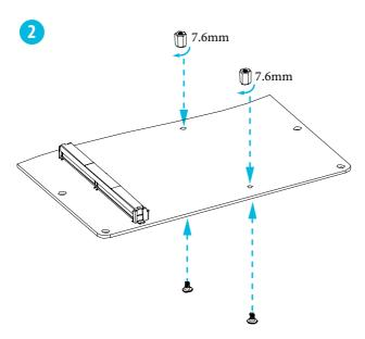
\*Before installing a Type B+ MXM card, please replace the 5mm standoffs with the 7.6mm standoffs.
