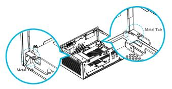
4. Refasten the two screws in the chassis.
