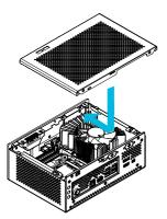
6. Refasten the four screws of the back panel.
