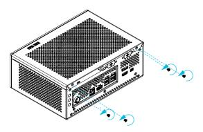
2. Slide the top cover outward and then lift it off the chassis.
