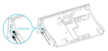
2. Fasten the screw nuts to secure the antenna connectors.
